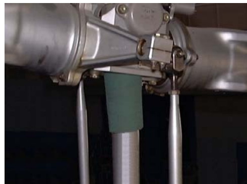
Figure 2. OH-58A/C Mast Wedge Assembly
