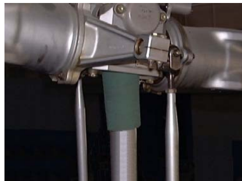
Figure 2. OH-58A/C Mast Wedge Assembly
